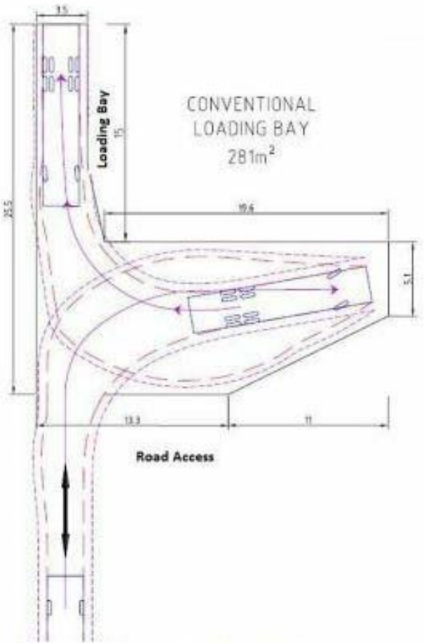
PENRITH COUNCIL TURNING CIRCLE DIAGRAM FORWARD & REVERSE
