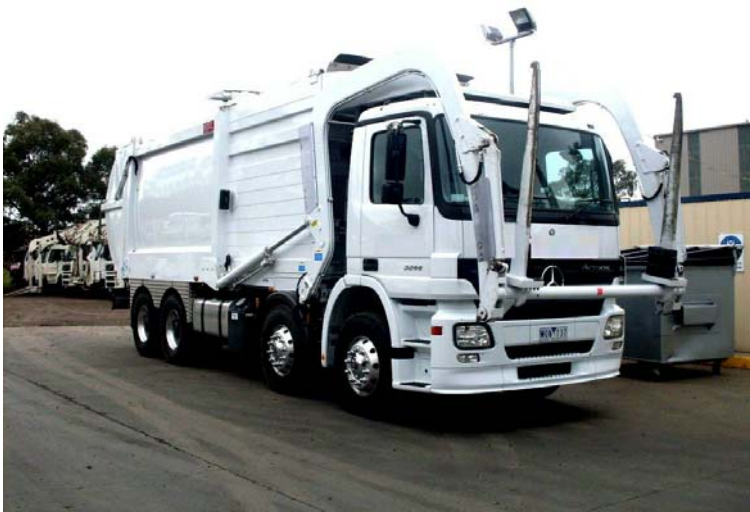
FRONT LOADER GARBAGE TRUCK 10.89M LONG 2.5M WIDE
