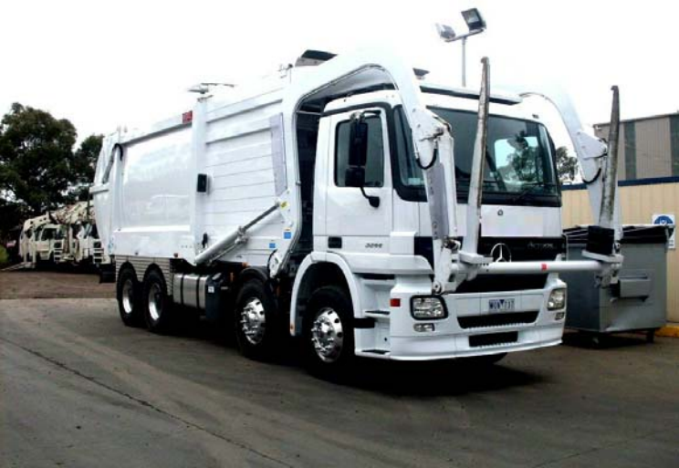
FRONT LOADER GARBAGE TRUCK 10.89M LONG 2.5M WIDE
